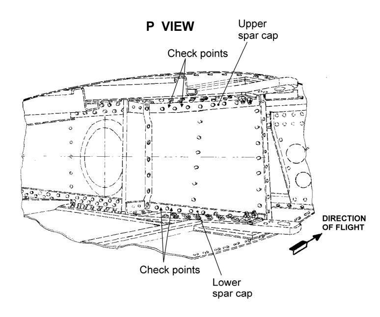
Fig. 2 - Check points on the upper and lower spar cap
